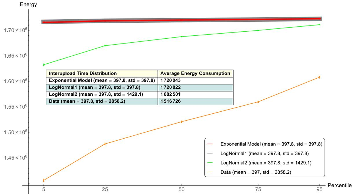
Fig. 2: Percentile and average values obtained for the 20 Apps scenario.
